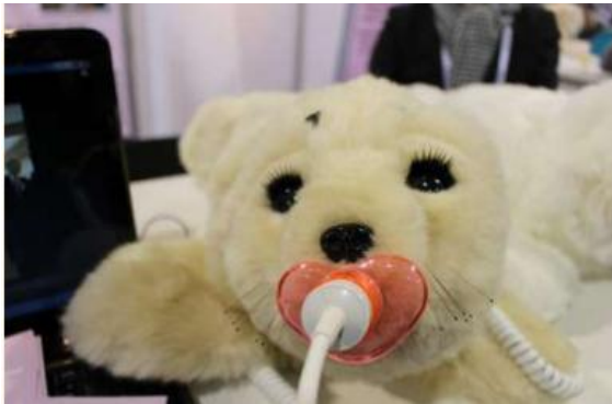
Figure 3. Paro, a psychotherapy seal robot developed by Japan Institute of industrial technology.
