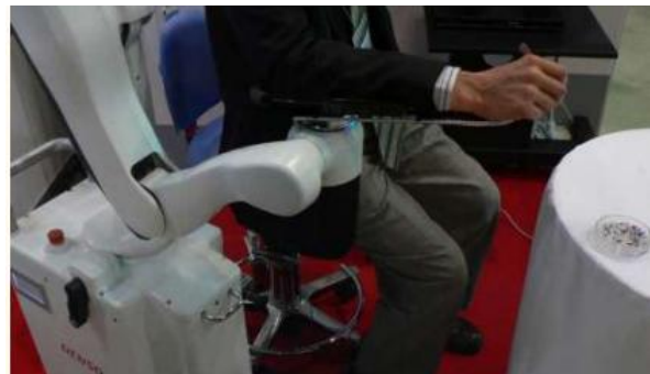
Figure 12. iArmS, an automatic tracking support arm launched by Japan Electric Equipment Company.
